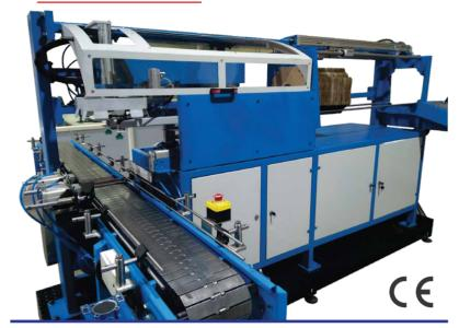
Stelda Automatic TCP 15 picks up corrugated from a stack applies hot melts adhesive and places it in top of a 15 Liter / 15kg tin containing edible oil. The machine is connected completely in line with oil filling plant, and the collar fixing operation is done at speeds synchronizing with the line speed.
